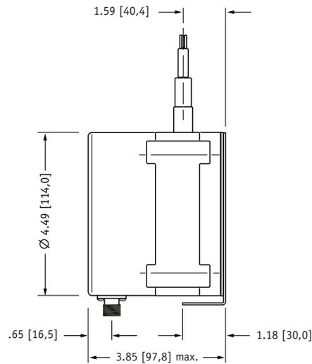
Fig. 3 - "Down" Cable Exit Direction
