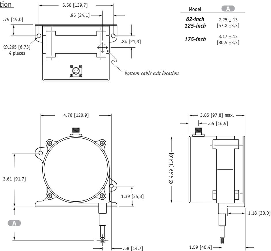
Fig. 4 - "Rear" Cable Exit Direction
